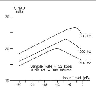
Figure 7: SINAD vs. Input Level at Different Frequencies
