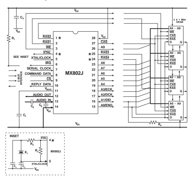
Figure 2: Recommended External Components
