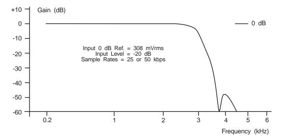
Figure 8: Typical Overall (Encoder + Decoder ) Frequency Response
