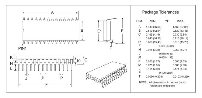
Figure 11: 28-pin CERDIP Mechanical Outline: Order as part no. MX802J
