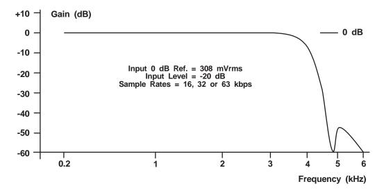
Figure 5: Typical Overall;; (Encoder + Decoder) Frequency Response
