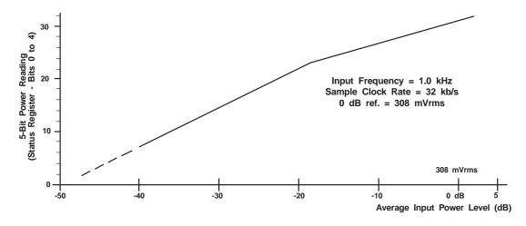
Figure 4: Typical Power Readings vs. Input Levels
