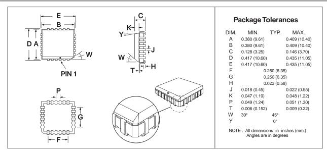
Figure 13: 24-pin PLCC Mechanical Outline: Order as part no. MX802LH
