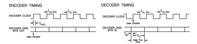
Figure 10: Codec Direct Access Timing
